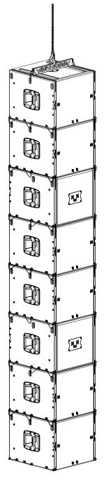
In some cases, asymmetric arrays are unavoidable, especially when the arrays are configured in blocks of four cabinets. In these cases, coverage tends to be biased towards a specific direction, but strategic placement can help shape coverage to the specific needs of a venue. Use LAC-3 to design such arrays.
